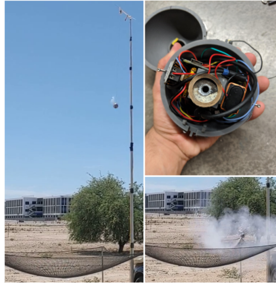
(b) (MS Thesis) Sensor node using two-axis spin stabilization (precession) for rocket motor exhaust vectoring, achieving soft touchdown at 10cm/s after an 8.7m drop. The system was designed for Lunar lava tube descent and mapping.
